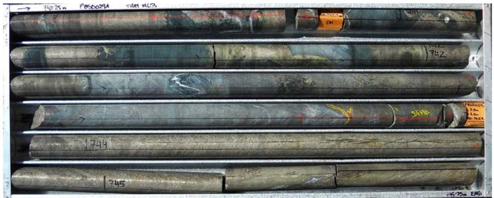
Figure 1: Golden Swan High-Grade Massive Nickel Sulphides
