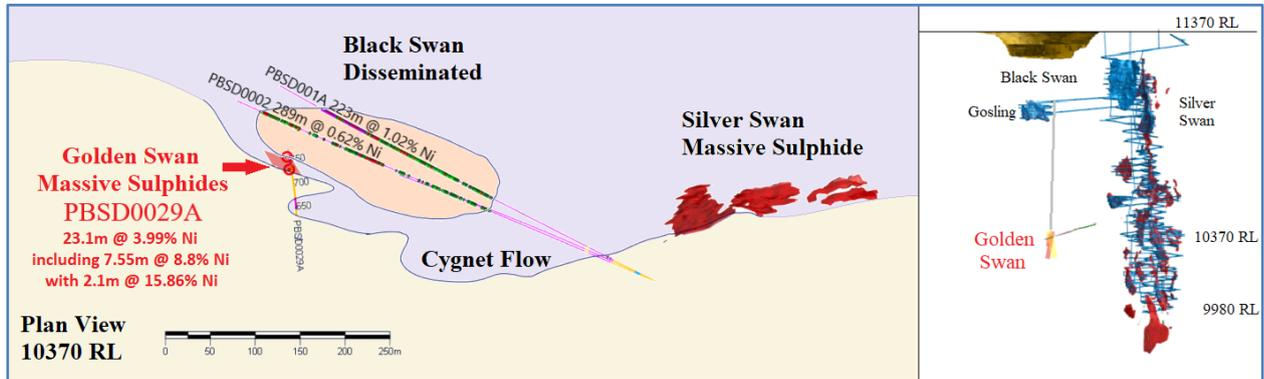
Figure 4: Interpretation of the blebby mineralised envelope (from 2019) and the location of the Golden Swan massive sulphide intersection. South is to the left.
