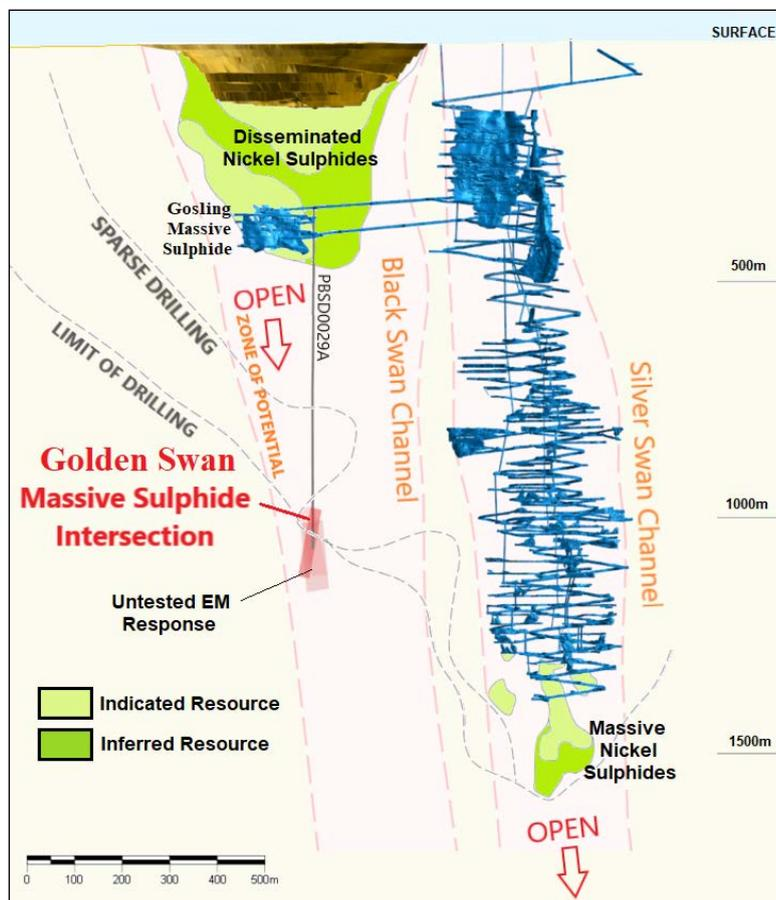
**Figure 2: Long section showing the Golden Swan massive nickel sulphide intersection and EM response within the Black Swan channel. The “zone of potential” for Gosling repeats and the upper limit of the Golden Swan massive sulphide will be EM tested by PBS0029A.**
