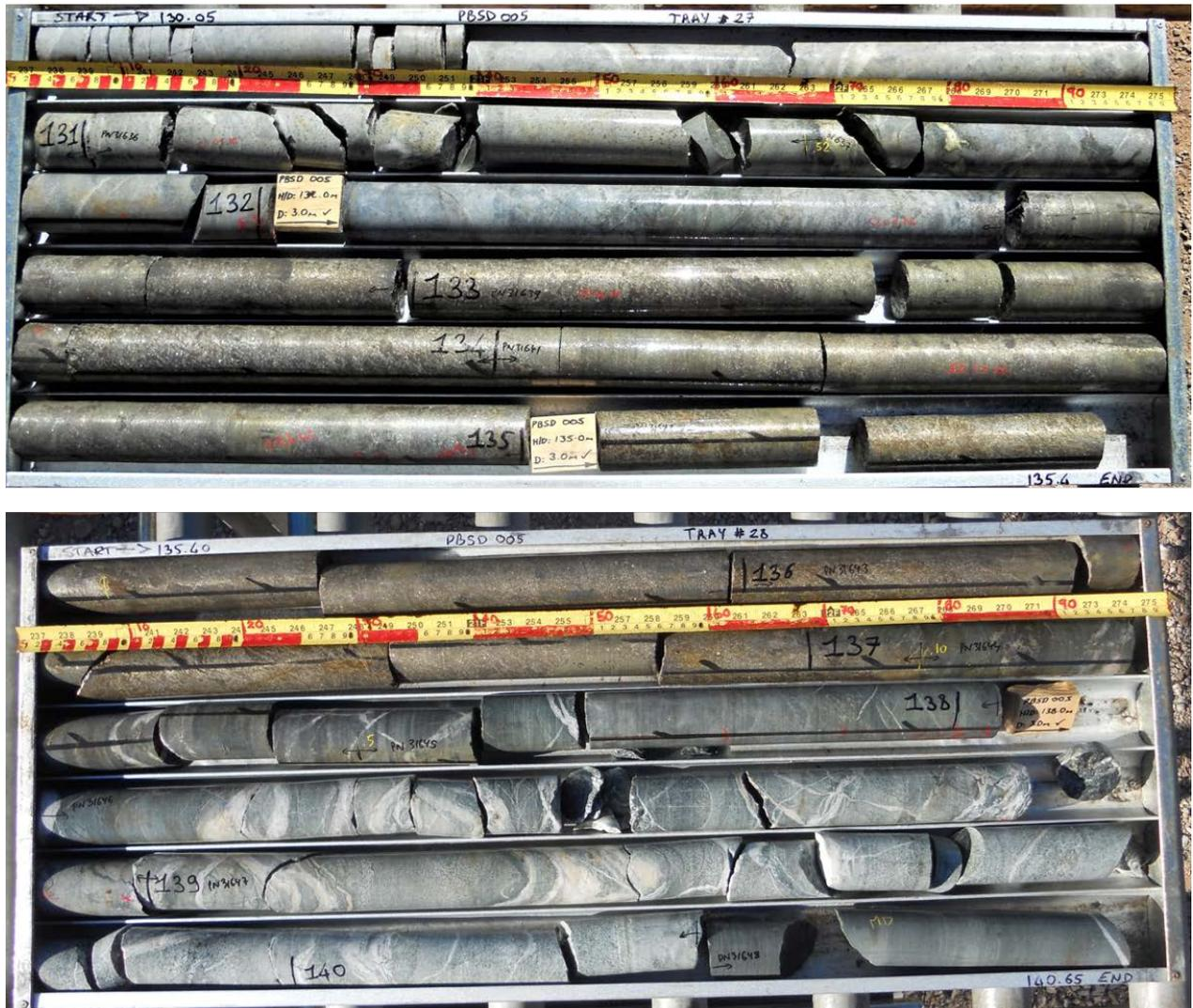
**Figure 1: Core from PBSD005 (Tray 27 & 28) showing massive sulphide mineralisation**
