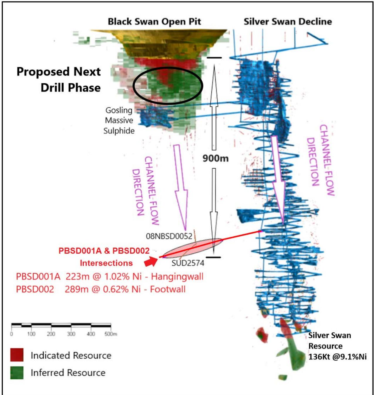
Figure 3: Longsection showing 2018 Resources and Black Swan Disseminated drill hole intercept location
