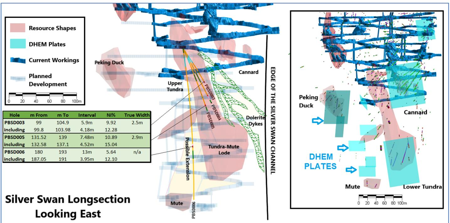
Figure 2: Silver Swan longsection - DHEM Plates and Drill Hole locations
