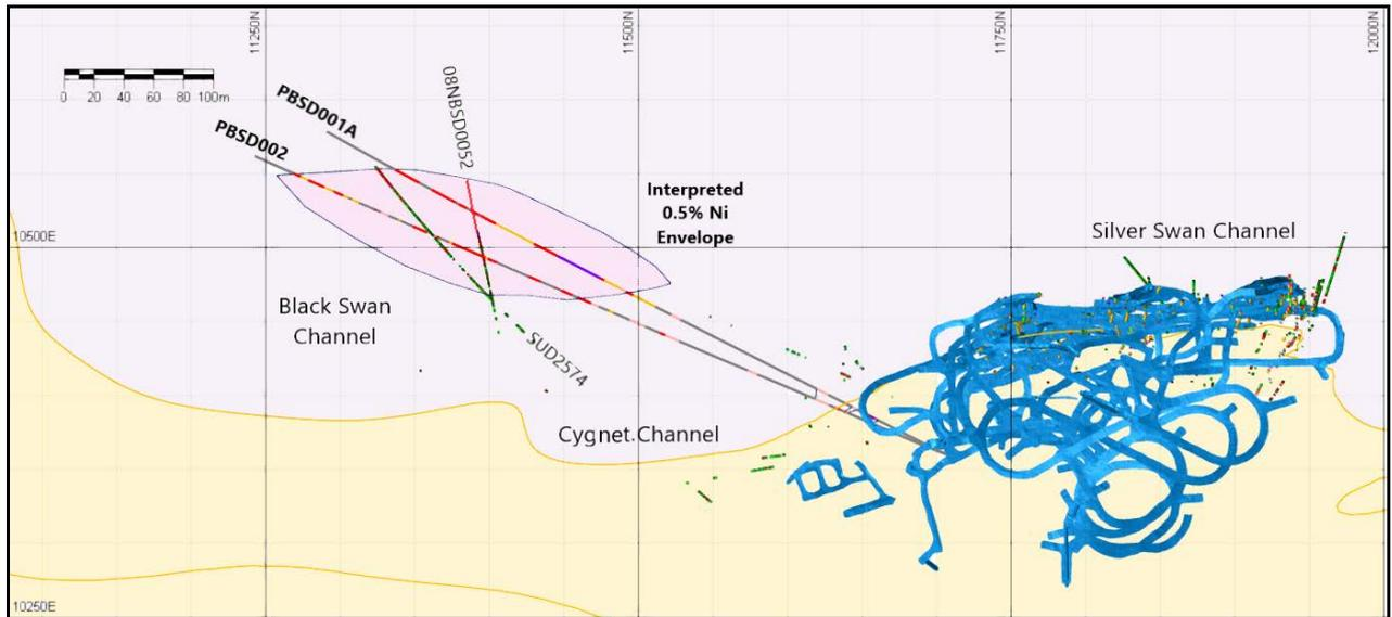
Figure 4: Plan view showing the PBSD001A and PBSD002 intersections in relation to historical drilling at one kilometre vertical depth below surface
