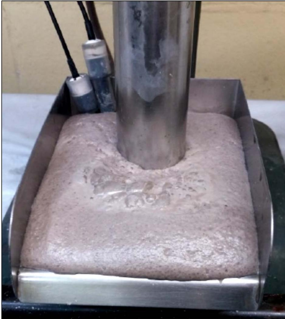
Figure 1: Pegmatite flotation test
