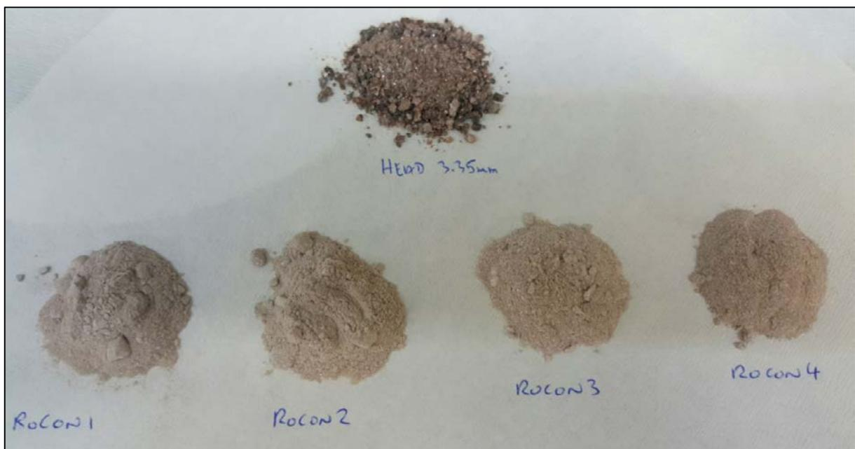
Figure 2: Initial head sample and concentrate recovered via flotation
