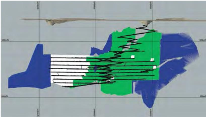
Figure 1: Maggie Hays Long-Section (Looking West), location of JORC Resources (green=Indicated, blue=Inferred), existing mining infrastructure (black) and mined out cave zone (white).
